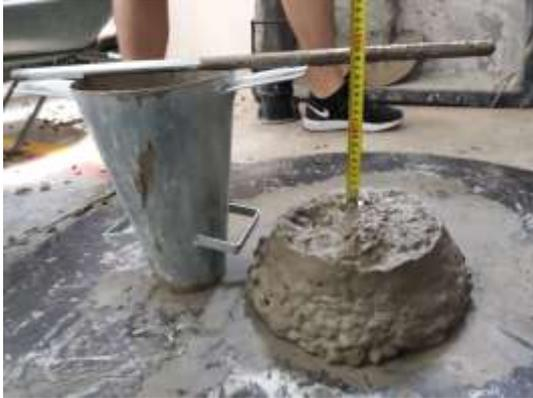
**Figura 8 – Slump test (CP2)**
