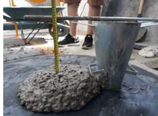
Figura 8 – Slump test (CP2)
