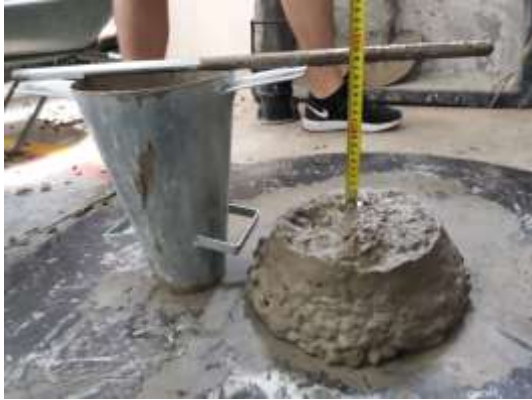
Figura 7 – Slump test (CP1)
